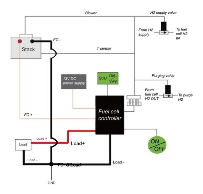
SCU: Short Circuit Unit GND: Grounding
