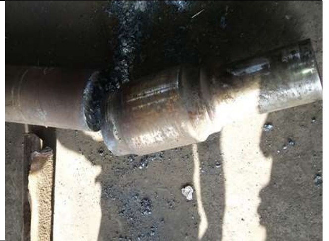
Axle cut by CNG.
