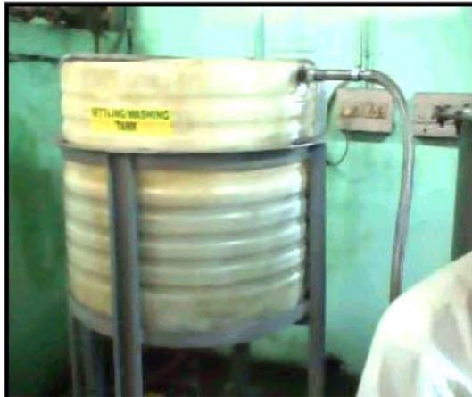
Figure 8 : Settling & washing tank
