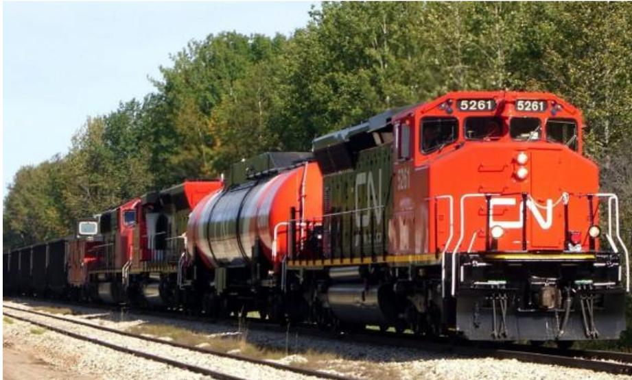
*The single LNG tender supports twin EMD SD40-2 locomotives with 16-645E3 engines, modified to run on an LNG-diesel mix using an ECI kit and key software. The fuel is vaporized on the tender and carried cross the couplers as a warmed gas.*
